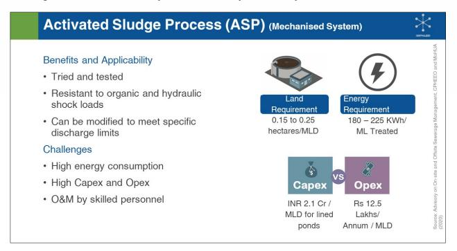
Treatment efficiency can be severely compromised if the plant is under- or over-dimensioned. Depending on the temperature, the solids retention time (SRT) in the reactor ranges from 3 to 5 days for BOD removal, to 3 to 18 days for nitrification. The excess sludge requires treatment to reduce its water and organic content and to obtain a stabilized product suitable for end-use or final disposal. It is important to consider this step in the planning phase of the treatment plant.
