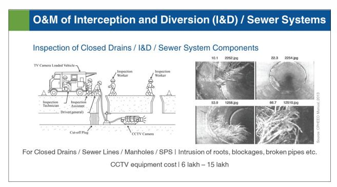
The closed drains with less than 3 ft width or sewer pipes with inside diameters ranging from 150 mm to 900 mm can be inspected by CCTV. The TV camera may be the traveling type or the towed type. Either the direct method (taking panoramic shots of the overall scene) or the side view method of taking local shots of only abnormal locations may be used.
