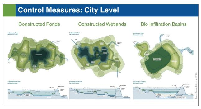
This slide shows three measure that can eb implemented at the city level for stormwater and combined sewer overflow management.
