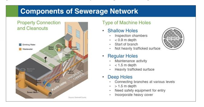
**Property connections and cleanout:** This is a vital component of any sewerage system. Without property connections, the system cannot be made functional. Property connection can be charged to the household as onetime fee, or spread over few years in the tax or can be subsidized or completely covered under the project. While providing household connection, plumbing must be below the level of water connection pipe and a cleanout shall be placed at appropriate place.
