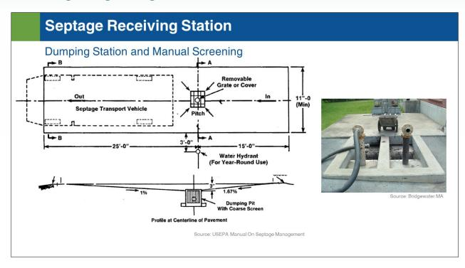
The aim of the septage receiving station is to reduce the impact and risk on STP due to co treatment of septage and sewage. Faecal sludge and septage receiving facilities provide the interface between FSS delivery vehicles and the sewage treatment plant. The aim of the facility is to allow for FSS transport vehicle access, providing adequate space for vehicles to discharge their contents and exit the treatment facility.
