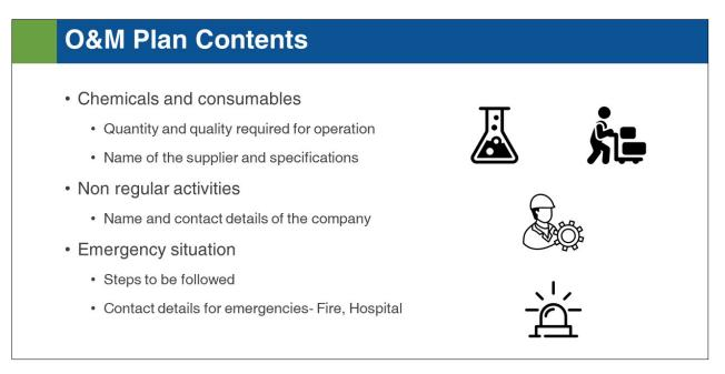
O&M plan should consist of consumables such as chemicals and their required quantities or dose, name of the supplier and its specification. Storage details of these consumables should also be mentioned. In case of non regular activities such as overhauling of equipment etc. name and contact details of the supplier or the technician shall be mentioned. The plan should also contain the steps that need to be taken in case of emergencies such as fire or medical emergency or natural calamity etc.
