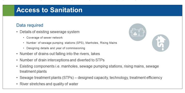
This slide includes the list of data sets required to understand the status of access to sanitation in the project area or at city level. The details of the existing sewerage system like coverage of sewer network, sewage pimping stations, manholes, rising mains, existing STPs need to be collected. The existing drains out falling into the surface water bodies i.e., rivers or lakes etc. also need to be monitored.
