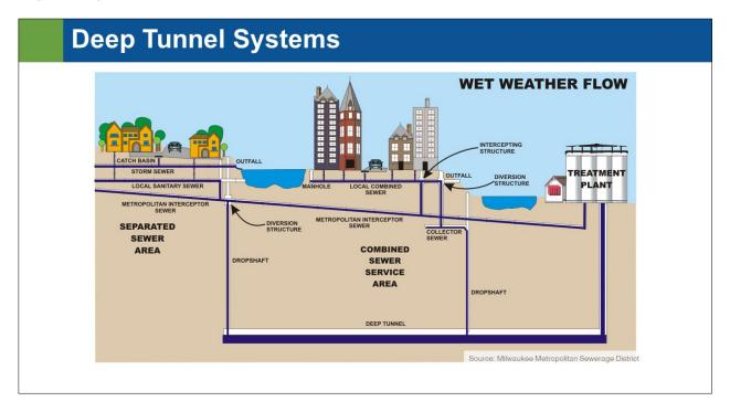
The engineering solution to reduce the overflows into the surface water body is deep tunnel or overflow surge tanks.
