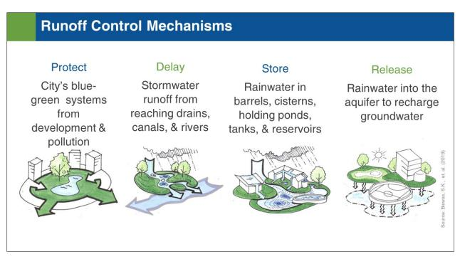
The slides show various runoff control mechanisms.
