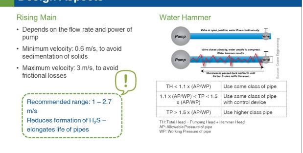
Pressurized pipe line after a lift station or a SPS is known as rising main. The design of rising main is critical as velocity of the wastewater needs to be maintained between 0.6 m/s and 3 m/s. The rising main should be as far as possible be laid with an even gradient with a minimum of sharp bends and curves.
