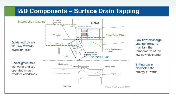
In case of I&D project on the surface drain, there are various components involved.
