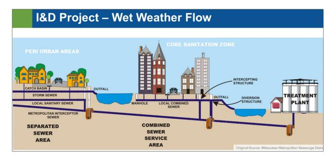
The picture represents the state of I&D project during the wet weather condition (i.e., high intensity rainfall). In peri urban areas, where separate sewers are implemented, only the stormwater will overflow in the surface water body. However, the combined sewer system in the CSZ will overflow into the surface water body once the interceptor sewer reaches its full capacity. Ideally, the I&D project should be so designed that this combined sewer overflow is restricted to four time in a year.
