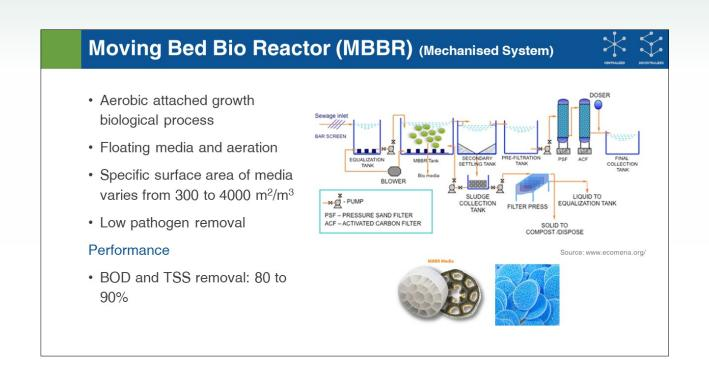
The MBBR is a complete mix, continuous flow through process which is based on the biofilms principle that combines the benefits of both the activated sludge process and conventional fixed film systems without their disadvantages.
