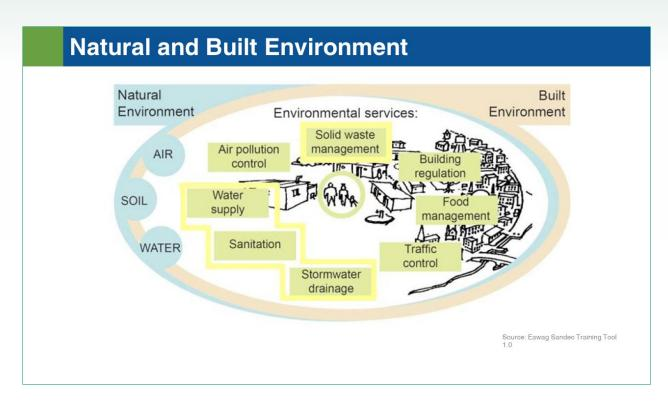
The natural and built environment with its natural resources water, air and soil (blue); all services and facilities required to keep the environment clean and protect health (green). WASH focuses on water supply and environmental sanitation services, facilities and human behaviour (inside yellow line).
