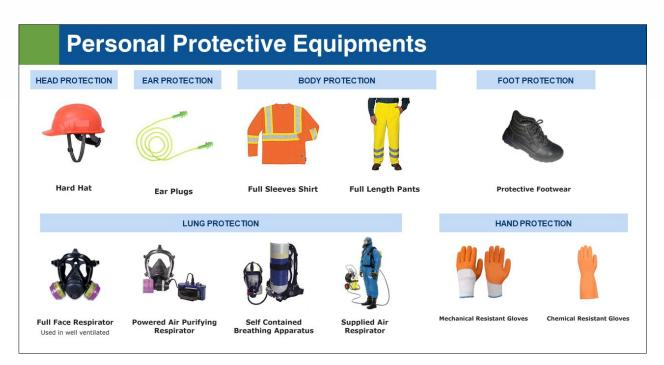
On your screen, you can see various personal protective equipments like hard hat, ear plugs, protective footwear, hand protection etc, which are required to safeguard health of the workers, during the cleaning of septic tank or sewer lines.
