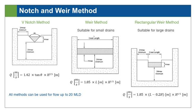
Notch and the Weir Method is more accurate as compared to the Float Method. It can be applied in any kind of drain of a pipe.
