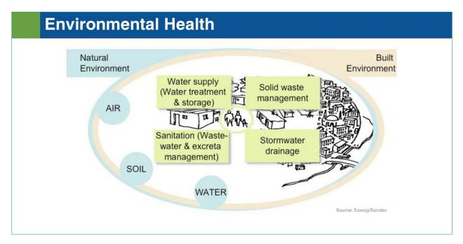
The water supply and environmental sanitation systems provide barriers between pollutants, the natural and built environment, and humans. The waste and resource sub-systems of water and environmental sanitation (green); the natural environment (blue); the built environment (brown).
