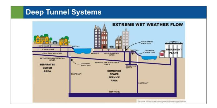
This slide shows that engineering solutions can also not provide a comprehensive solution. In case of storm like event, the deep tunnel or surge tank might reach to its capacity and overflow can still take place. Thus, it is essential, that stormwater management is promoted at various levels – household, community and city.
