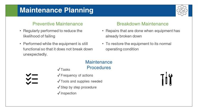
Maintenance procedures are of two types- Preventive maintenance and Breakdown maintenance.
