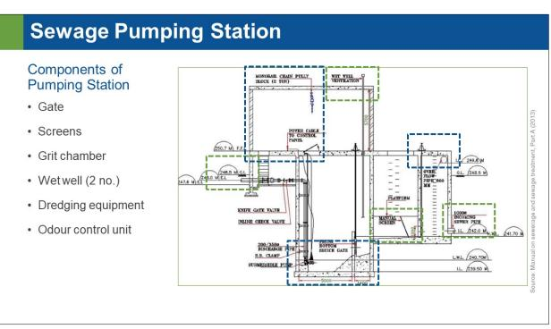
Sewage Pumping Station (SPS) handle sewage either as in-line for pumping the sewage from a deep sewer to a shallow sewer or for conveying to the STP or outfall. They are required where sewage from low lying development areas is unable to be drained by gravity to existing sewerage infrastructure, and / or where development areas are too remote from available sewerage infrastructure to be linked by gravity means. SPS consist of different components as shown in the picture.
