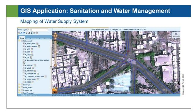
This slide represents the application of GIS in water and sanitation management while providing essential environmental services to the citizens. It represents the integration of water supply system dataset i.e., water supply pipelines, junctions, water meters, water treatment plants etc. with the georeferenced spatial data inform of thematic map (Source: GIS Portal, Surat Municipal Corporation)
