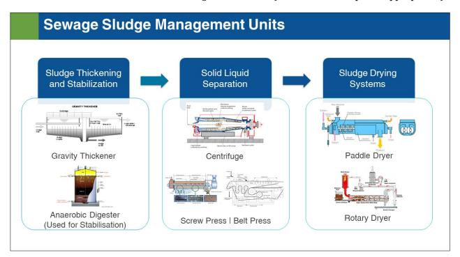
Solid liquid separation is an important step in sludge handling at faecal sludge treatment facility or at co-treatment facility. After solid liquid separation, the semi thickened sludge has transferred to further sludge handling facility and liquid has be transferred to liquid treatment system. It has two different approaches natural system (i.e., settling thickening tank etc.) or mechanized system (i.e., by mechanical presses like screw press or belt press etc.)
