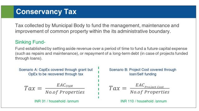
Conservancy tax is a tax collected by municipal body to funds the complete project or O&M of the project over its life time. It can be calculated using the formula given in the slide. Since, the tax is based on the EAC, its collection for initial few years will lead to higher revenue than needed. This extra revenue shall be deposited in the sinking fund. The amount in sinking fund earn interest and supports the O&M cost in the later year when the annual O&M cost is more than the tax collected.
