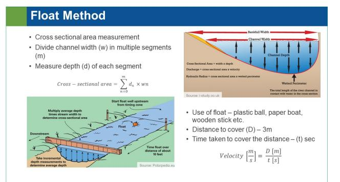
Float Method consists of two stages: (1) Stage 1: Measuring the cross section of the drains and (2) Stage 2: Measuring the time taken by a float to cover a predetermined distance in the drain.
