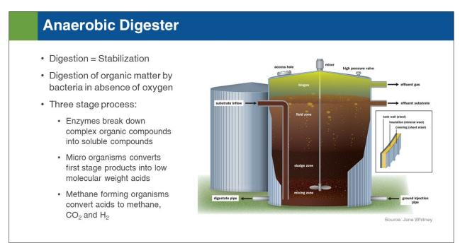
Anaerobic digester provides stabilization of sludge by digesting the volatile solids using bacteria in absence of oxygen. Anaerobic digestion is a three-stage process: (1) The enzymes break down the complex organic compounds in the soluble compounds. This mainly happens through hydrolysis process. (2) In the second stage the soluble compounds are converted into low molecular weight
