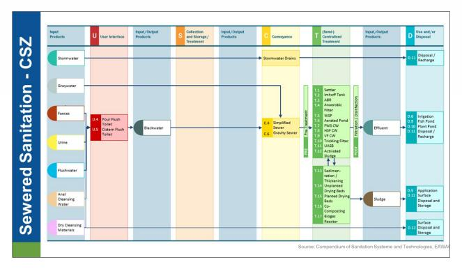
This is a water-based sewer system in which blackwater is transported to a centralized or semicentralized treatment facility. The important characteristic of this system is that there is no collection and storage/treatment (also known as containment unit). Inputs to the system include faeces, urine, flush water, anal cleansing water, dry cleansing materials, greywater and possibly stormwater.
