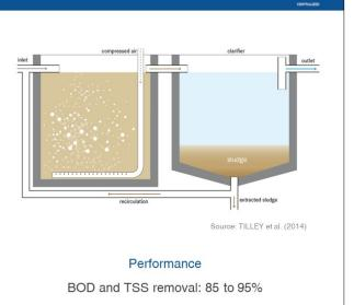
An activated sludge process refers to a multi-chamber reactor unit that makes use of highly concentrated microorganisms to degrade organics and remove nutrients from wastewater to produce a high-quality effluent. To maintain aerobic conditions and to keep the activated sludge suspended, a continuous and well-timed supply of oxygen is required.
