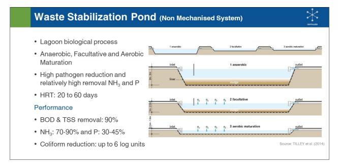
Waste Stabilization Ponds (WSPs) are large, manmade water bodies. The ponds can be used individually, or linked in a series for improved treatment. There are three types of ponds: (1) anaerobic, (2) facultative and (3) aerobic (maturation), each with different treatment and design characteristics.
