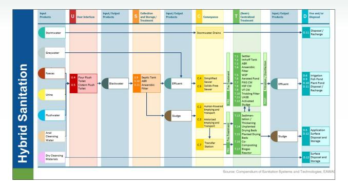
This system is characterized by the use of a containment unit such as a septic tank (also known as interceptor tank) and the household level to arrest settleable solids from the blackwater, and a simplified or solids-free sewer system to transport the effluent to a (semi-) centralized treatment facility. Inputs to the system can include faeces, urine, flush water, anal cleansing water, dry cleansing materials and greywater.
