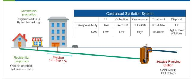
**Conventional gravity sewers** are large networks of underground pipes that convey blackwater, greywater and, in many cases, stormwater from individual households to a (Semi-Centralized Treatment facility, using gravity (and pumps when necessary).
