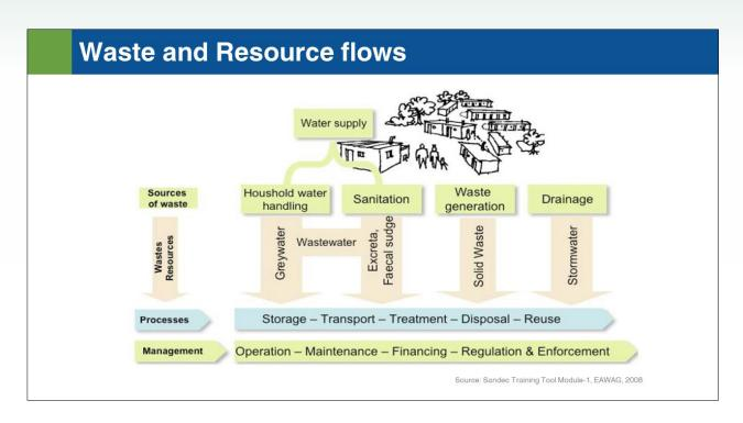
The figure shows the sources of waste in the household and neighbourhood (green) and the waste and resource flows (brown). All waste and resource flows require an integrated management (green) within a settlement: regulatory system and its enforcement, as well as operation and maintenance for safe transport, treatment, safe disposal, and/or reuse (blue).
