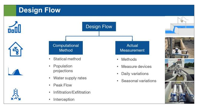
Design flow can be estimated using two methods: (a) computational method and (b) actual measurement. The computation method is based on the statistical information and assumptions whereas the actual measurements indicate the actual flow in the drain/pipe at the specific time of the day.
