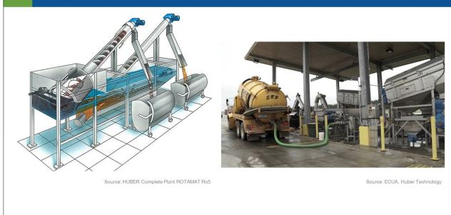
It represents the mechanized system for the septage receiving station which includes the dumping site, mechanized screening system and mechanized longitudinal grit trap. Integrated pretreatment module combines the mechanical screen and longitudinal grit trap. This is a single equipment which can be placed after the dumping station. Washing, and dewatering is optional and is recommended so that the solid waste and grit can be safely handled and disposed appropriately.
