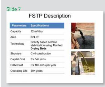
The treatment plant is based on a very simple technology of planted drying bed in which sludge is treated using evapotranspiration from plants, which are planted on the sludge drying bed.
