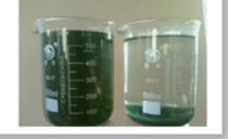
Coagulation/flocculation is the process of adding chemical enhancers in order to increase the sedimentation. This is done prior to dewatering so that the process becomes more convenient.
