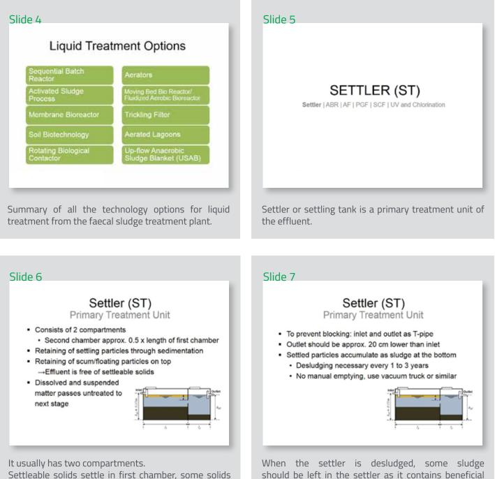
Settleable solids settle in first chamber, some solids move to second chamber and settle there.
