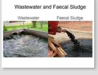
Wastewater is different from faecal sludge in terms of source and characteristics. Fecal sludge comes from an on-site sanitation technology, whereas wastewater is transported through a sewered system.
