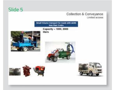
Containment systems along smaller road which can be accessed by smaller vehicles can be desludged using smaller mechanized equipments as shown in the slide.
