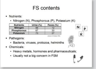
Faecal sludge is a rich source of nutrients such as nitrogen, phosphorous and potassium. But at the same time they consist of a host of pathogens and at time chemicals.
