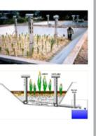
Planted drying bed dewaters the sludge using two methods of evaporation and evapotranspiration by means of plants. The bed consists of gravel/ sand/ soil filter through which the liquid flows vertically downwards and is collected and treated separately. This process helps in dewatering the sludge faster.
