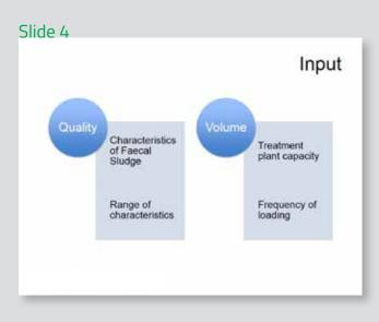
Input to a FSTP system can be classified under two buckets: Quantity and quality of the sludge.
