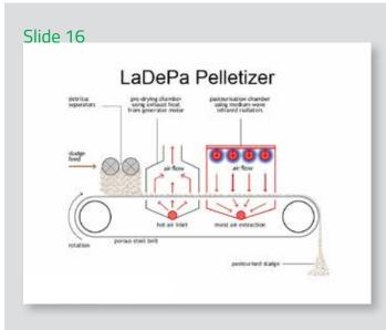
Schematic showing the working of a LaDePa pelletizer
