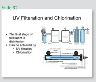
Final step in the treatment process is UV filtration and chlorination in order to ensure disinfection.
