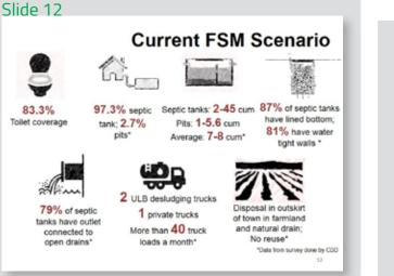
Due to the high water table, most of the containment units in the town are water tight septic tanks. In case of septic tanks, in 79% cases the effluent is let out into drains directly. When desludged, the faecal sludge is directly disposed of into the environment. <section-header><section-header><section-header><complex-block><image><image><image><image><image><image>
