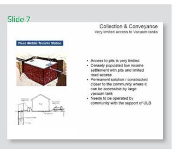
A sludge transfer station can work along with a cesspool vehicle by providing the vehicle access to inaccessible containment units.
