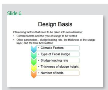
List of influencing factors which affect the design of an unplanted drying bed can be seen above.
