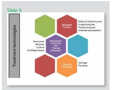
Mechanism of treatment technologies that are available for the treatment of faecal sludge can be categorized into following:
