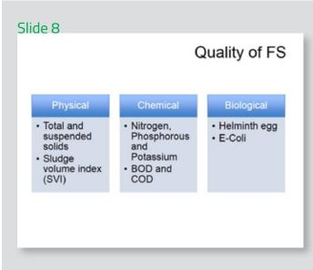
Quality of FS is bucketed under Physical, Chemical and Biological parameters which are crucial for deciding the type of treatment system required.
