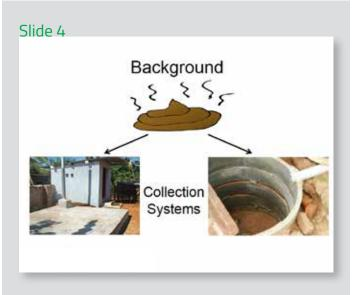
Faecal sludge is the excreta-derived sludge collected from containment systems such as pits and septic tanks.
