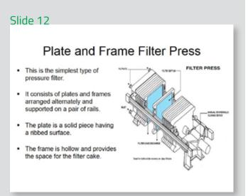
Construction and working of a plate and frame filter press for mechanical dewatering.
