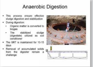
Anaerobic digestion is a biological treatment technology which is applicable for temperate and tropical regions. It is used to reduce the organic load by means of sludge digestion and stabilization.
