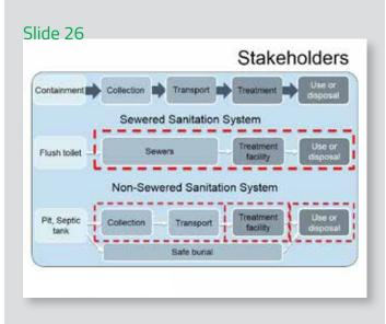
In case of sewered sanitation, the sewers, treatment facility and disposal mechanism acts as a single entity working closely with each other. Usually, all three are managed by one single agency.
