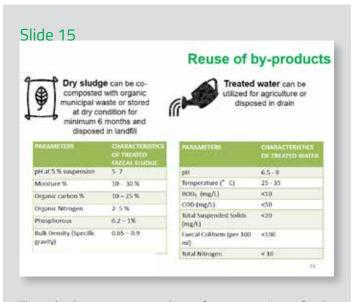
Though there are a number of reuse options for by products and the end products of an FSTP, the most popular one is the agriculture reuse in which the biosolids are co-composted with wet waste and used as a soil conditioner while the treated effluent is used for landscaping.
