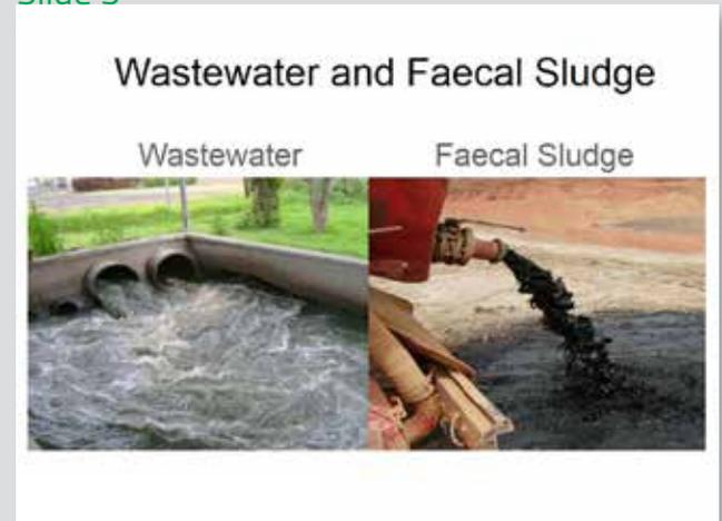
Wastewater is different from faecal sludge in terms of source and characteristics. Faecal sludge comes from an on-site sanitation technology, whereas wastewater is transported through a sewer system. Therefore, the treatment infrastructure will be different for each of them.
