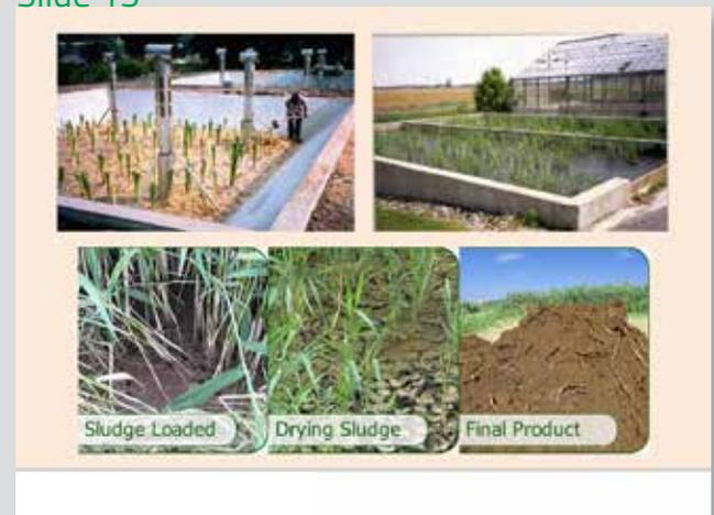
Pictures of the various stages of the operation of the planted drying beds.
