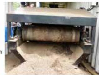
LaDePa Pelletizer uses thermal treatment. The machine works on the pyrolysis process which decomposes matters using heat in the absence of oxygen. Although it is energy intensive, a part of the energy can be provided by the pellets created from faecal sludge. For more information refer to FSM Book (Strande, Ronteltap, & Brdjanovic, 2014).
