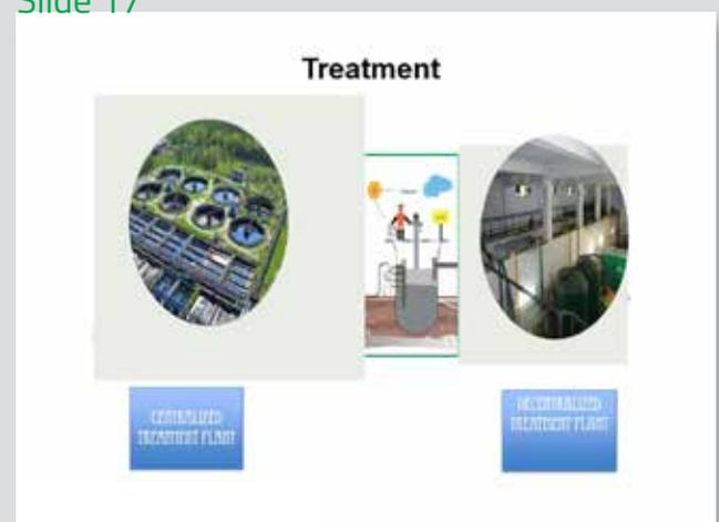
Faeces is treated in treatment plant which are centralized (catering to an entire town) and decentralized (catering to small pockets within the town, closer to the source of generation) in nature.
