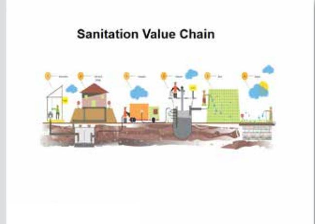
The sanitation value chain is a diagrammatic representation of the movement of faeces from generation to disposal. It has six components:
