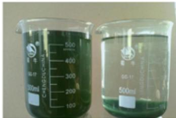
Coagulation/flocculation is the process of adding chemical enhancers in order to increase the sedimentation. This is done prior to dewatering so that the process becomes more convenient.
