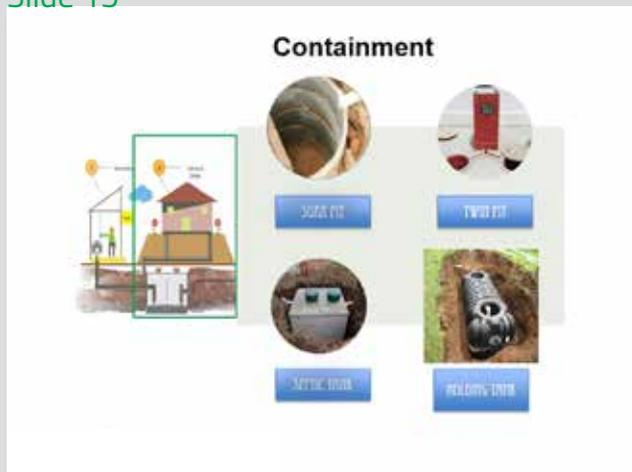
Containment or collection & storage comprises of the containment system. There are 4 common types of containment system:
