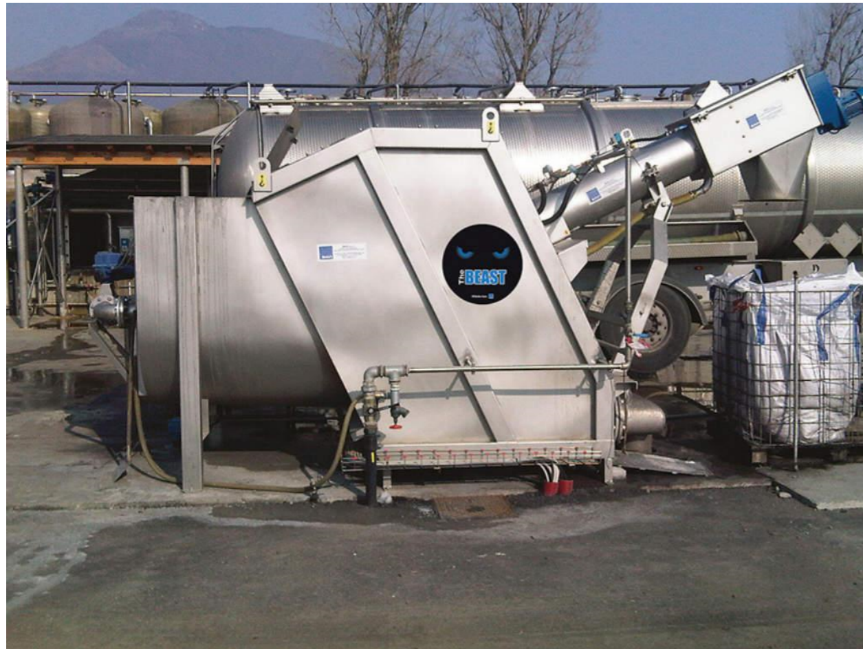
Figure 36: Picture of a prefabricated mechanical screen
