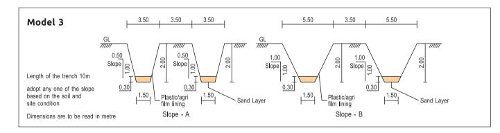
Construction of deep trench with sand barrier and plastic/agri-film is similar to normal deep trench and the dimensions are same (bottom width as 1.50 m and depth as 2.00 m, the side slope can be maintained as 0.50:1 or 1:1 depending on the soil type in the project location, if it is a hard formation 0.50:1 can be adopted and in case of loose formation, the side slope of 1:1 can be followed). The difference is that at the bottom of the
