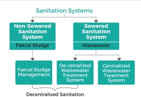
comprises of sewers to convey domestic wastewater from a neighbourhood or local catchment to a small, local treatment plant where it is treated through a natural processes without any requirement for external energy to operate the system.
