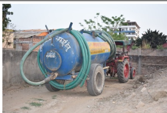
Private desludging Tanker
