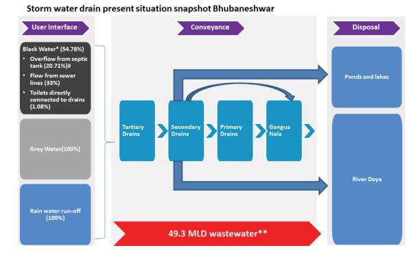
Figure 13: Storm water Drainage snapshot- Bhubaneswar Municipal Corporation
