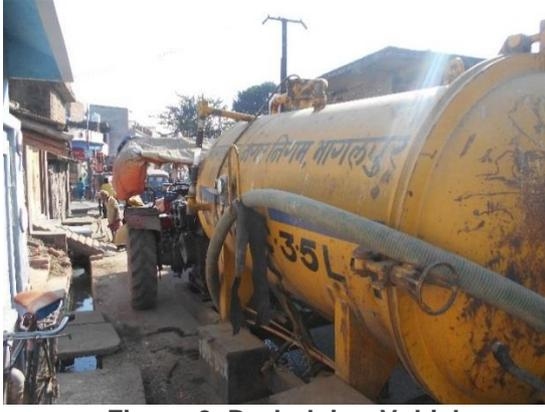
Figure 2: Desludging Vehicle
