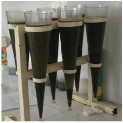
Figure 16 Imhoff cones being used in analyses of sludge volume index (Source: SANDEC).
