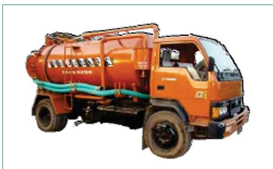
Figure 19: Truck mounted tanker
