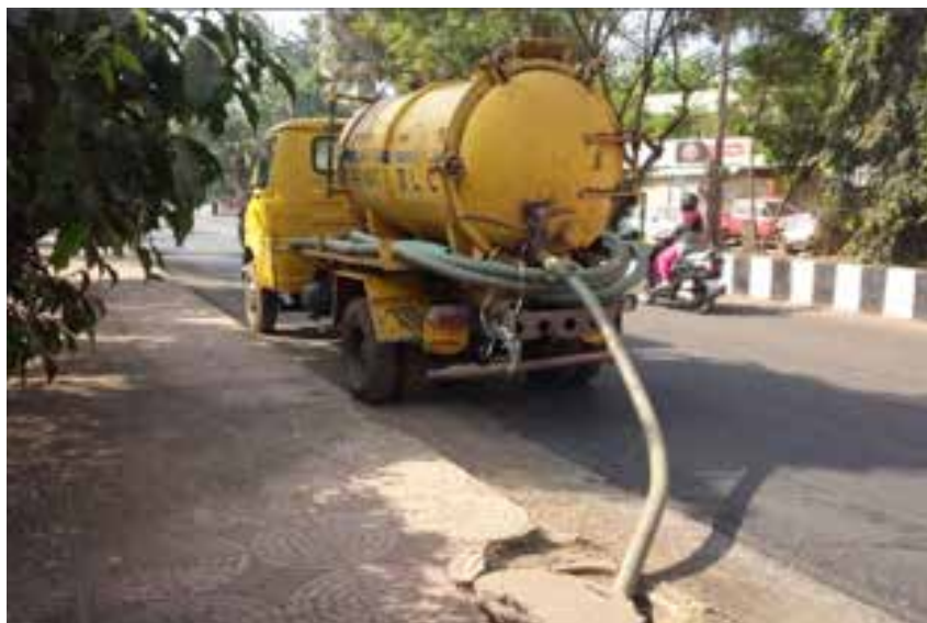
Figure 7: A Honeysucker Discharging Faecal Sludge Into The UGD
