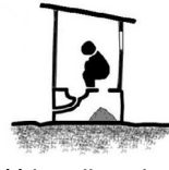
Urine diversion dehydration toilet
