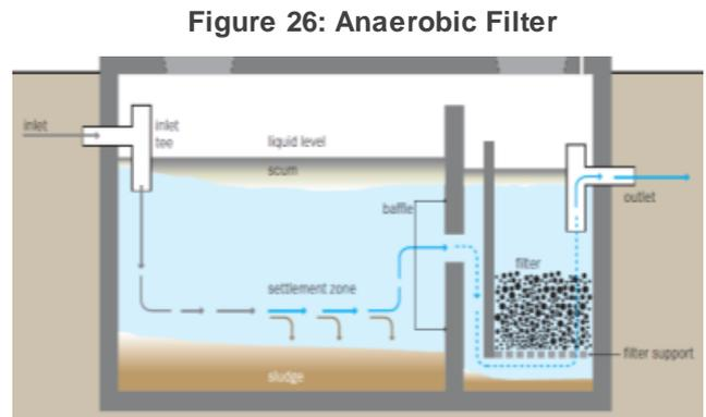
An important design criterion is equal distribution of wastewater upon the filter area. The baffle walls or pipes ensure the direction of wastewater flow within the tank; it forces the wastewater to flow through the filter media in each chamber. Each of the chambers is designed to take care of the required hydraulic and organic loading. Through intensive contact between wastewater and bacterial biomass, organic matter is digested with short retention times. The HRT of the tank will be 12-36 hrs.
