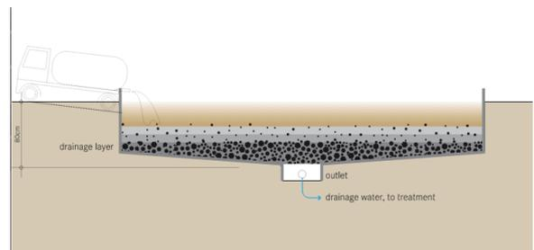
Figure 23: Sludge Drying Beds
