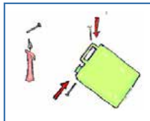
Make 2 holes with warm nail into plastic canister
