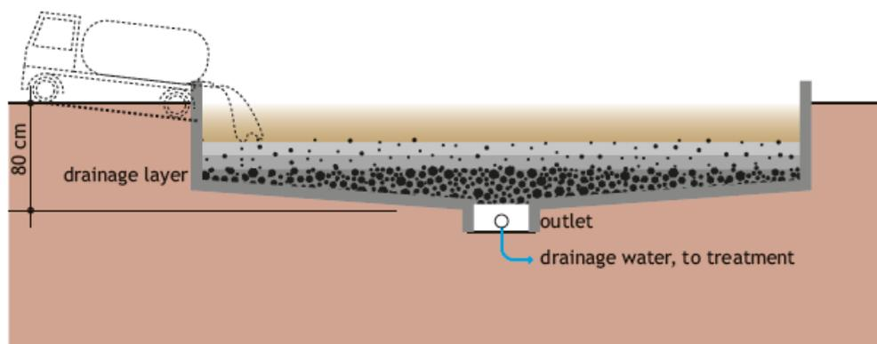
Figure 22 Schematic overview of an unplanted sludge drying bed (Tilley et al., 2014). A splash plate is not visible
