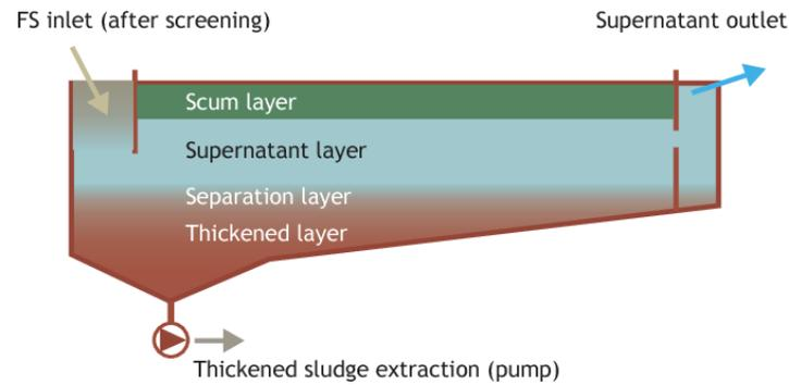
Figure 14 Schematic of the zones in a settling-thickening tank.
