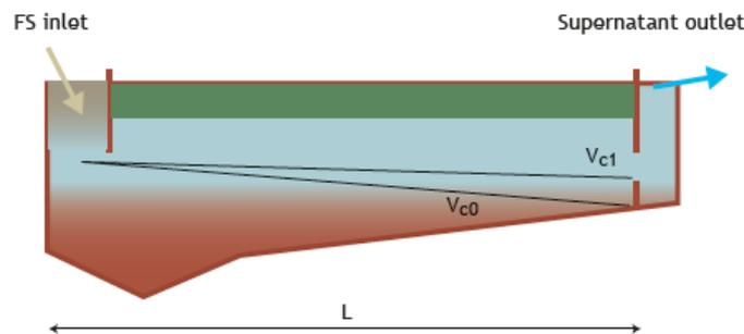
Figure 15 Schematic of the final settling velocity ( $V_c$ ) needed for a particle to settle in a tank of length  $L$ . (Source: Magalie Bassan et al)
