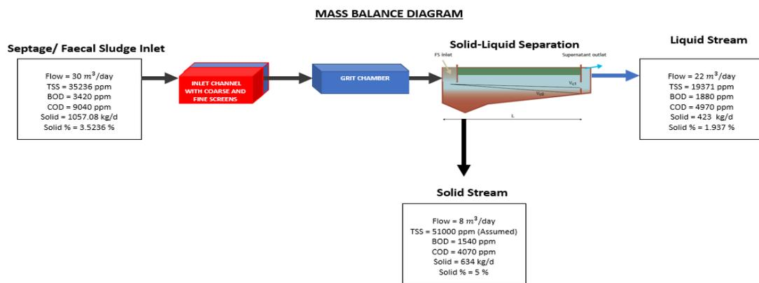
Figure 17 Mass flow diagram post solid-liquid separation
