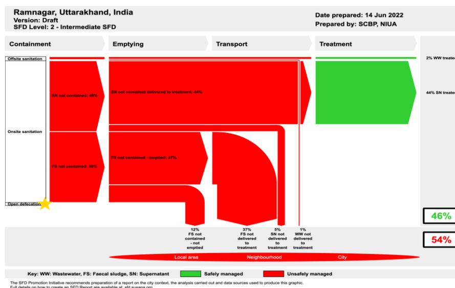
Figure 2 Shit flow diagram of Ramnagar (Source: Graphic Generator Sfd.Susana.org)
