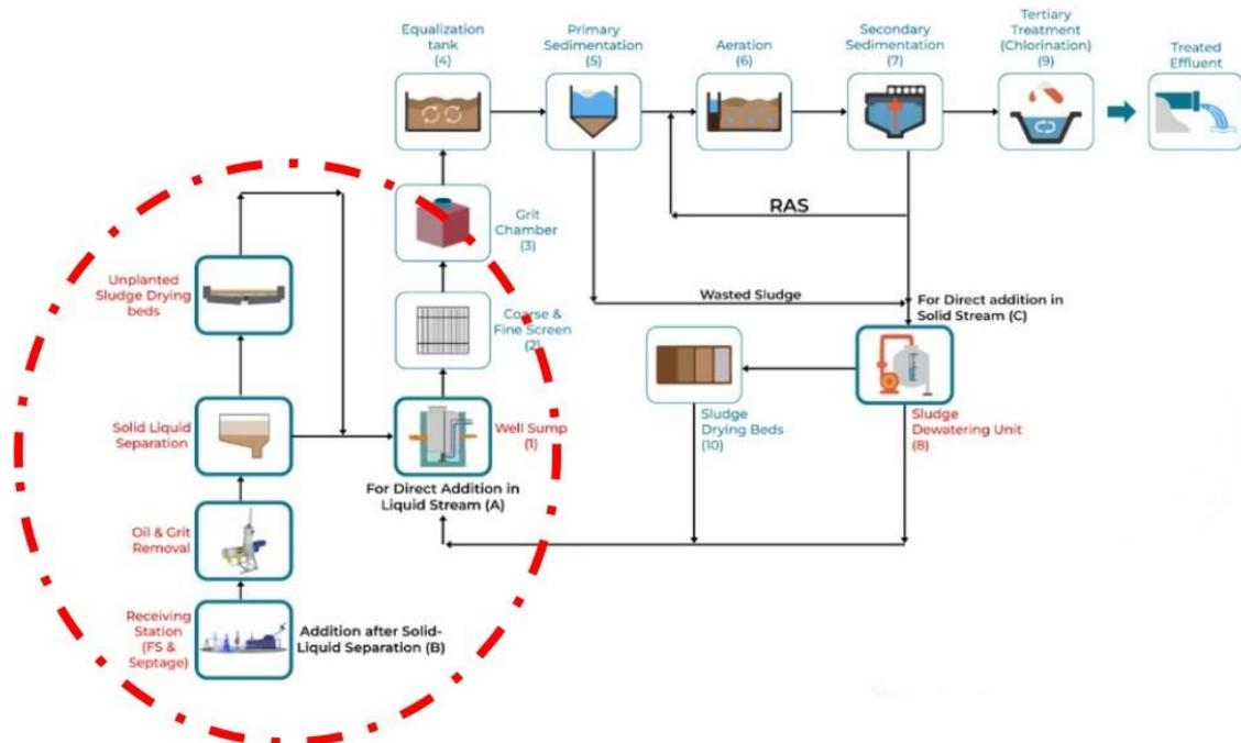
Figure 13 Process flow diagram depicting Co-treatment at the STP
