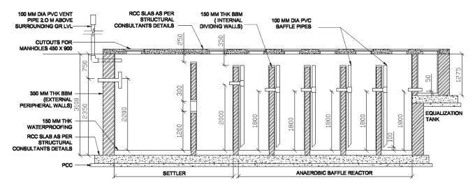
By means of the baffles, the water is forced to come in contact with the anaerobic bacteria which lives in the sludge located at the bottom of the thanks. Some turbulence is needed, but if the up velocity is too high, the water will pass through too quick reducing the efficiency of the treatment and flushing out the bacteria.
