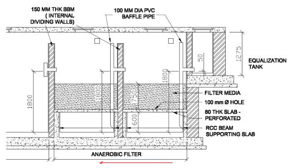
Filter material, such as gravel, rocks, cinder or specially formed plastic pieces provide additional surface area for bacteria to settle and grow. In fact, anything that can give more surface to the bacteria to grow will do. The fresh wastewater is forced to come in contact with active bacteria intensively. Actually, the larger the surface provided for bacterial growth, the quicker the digestion.
