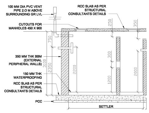
The Hydraulic Retention Time (HRT) is 1.5-2 hours. The settled solids are partially decomposed due to anaerobic condition and form sludge and collect at the bottom. Grease and light particles floats and form a thin layer at the surface of the wastewater referred to as scum.
