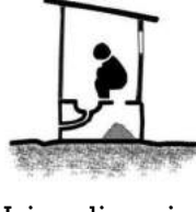
Urine diversion dehydration toilet
