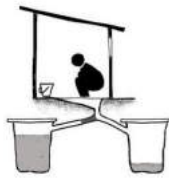
Twin pit for flush toilet
