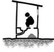
Urine diversion dehydration toilet
