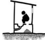
Urine diversion dehydration toilet
